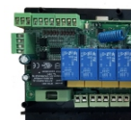
MPC-851 Motor/Power Controller with Radio Frequency Receiver
