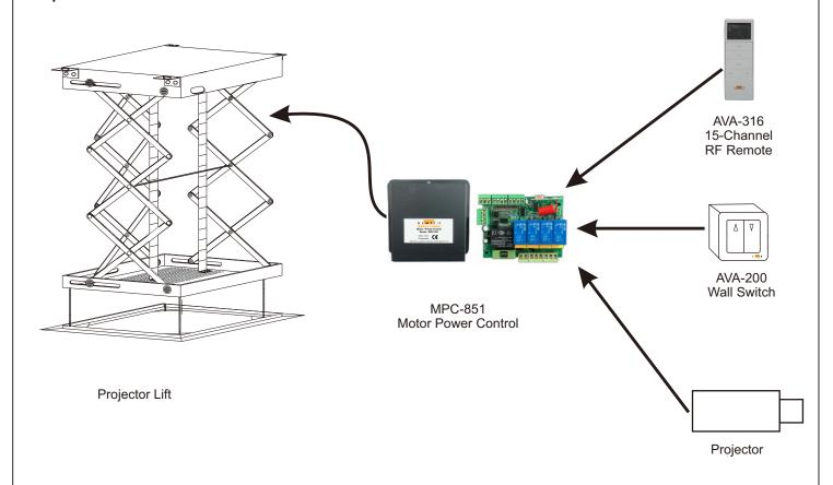
△ Connection of all cables to the MPC-851 (Refer to Installation Guide of MPC-851)
