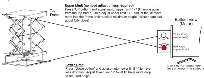
Do not adjust the Upper Limit of the lift higher than the original factory preset position. If adjusted, the lift will move into the frame and be stopped by force and not the Upper Limit Switch. This will cause overheating of the motor, rendering the lift to being unable to operate properly.
