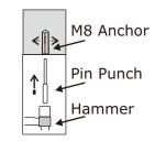
B) Insert M8 anchor into the hole. C) Use pin punch to expand the anchor.
