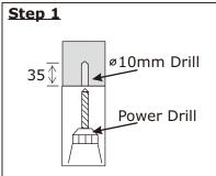
A) Drill Dia. 10mm holes to a depth of 35mm. (Note: Do not drill too deep)
