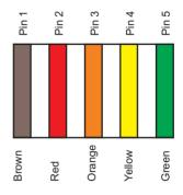
Brown = pin 1 Red = pin 2 Orange = pin 3 Yellow = pin 4 Green = pin 5 To control movement of the motorized lifter
